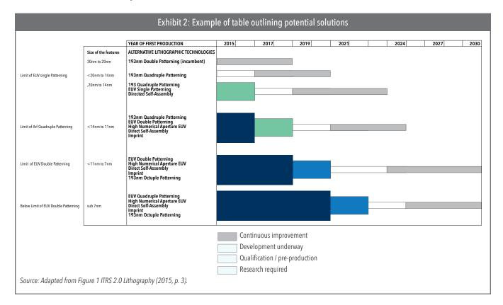
Exhibit 2 is an example of the information graphic used to show *potential solutions* for each technology that is part of the wafer production process. This exhibit presents the possible technology solutions for the lithography. In the semiconductor industry lithography refers to the processes that are used to print patterns on wafer chips.
